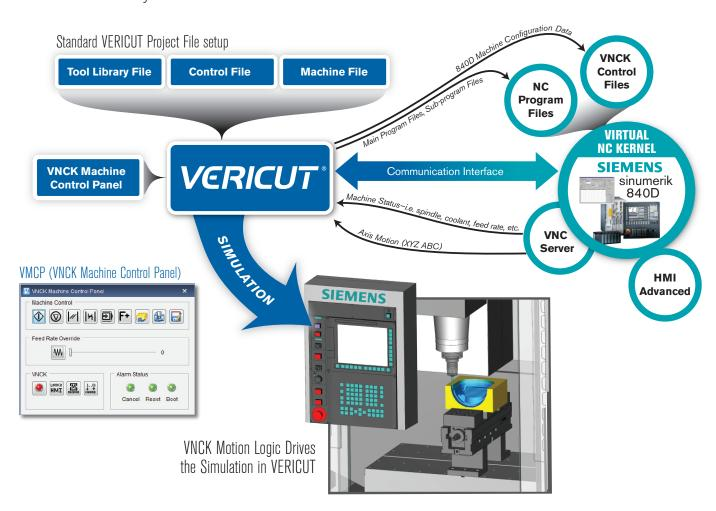
VERICUT CNC Machine Simulation software is integrated with the CNC motion logic of the Siemens SINUMERIK 840D control using Siemens' Virtual NC Kernel (VNCK).
