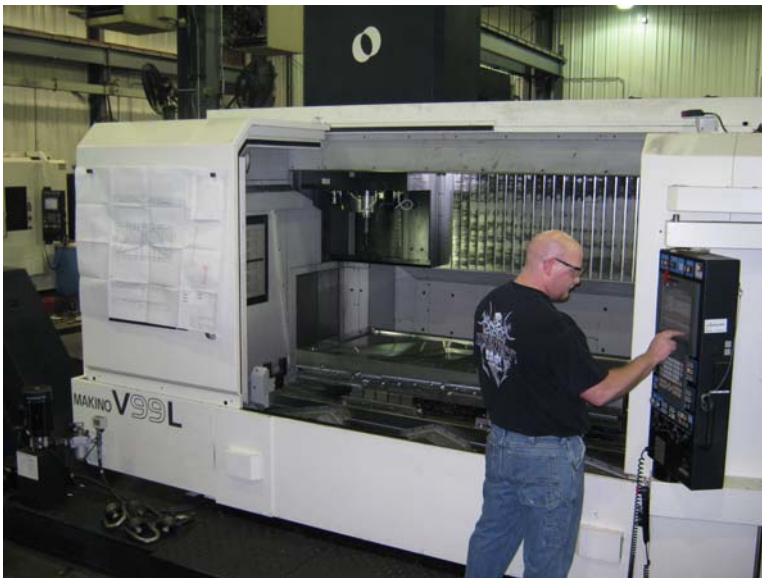
Operator Chris Wamser setting up the A-plate in the Makino V99L
