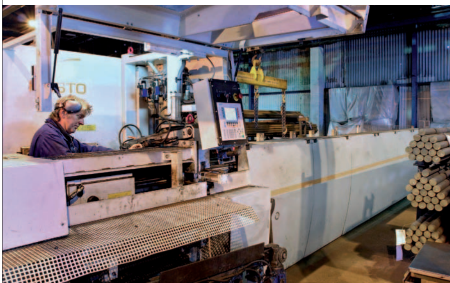
Top, Banks Precision uses its Okuma's Turn Cut facility; above, Cooper and Turner is using Kasto saw technology to cut fasteners accurately to length in support of the wind energy sector
